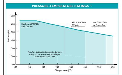
This chart displays the pressure-temperature ratings for the valve's body per ASME B16.42-1998.
